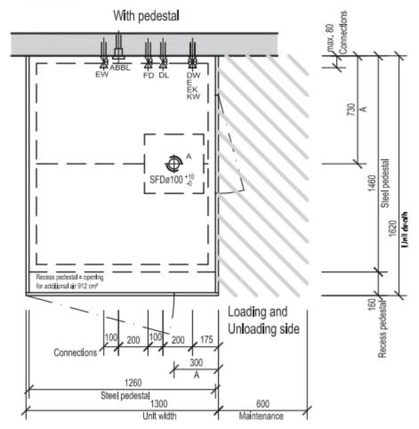
Integrated steam supply, steel pedestal or feets and side panelling are accessoires
